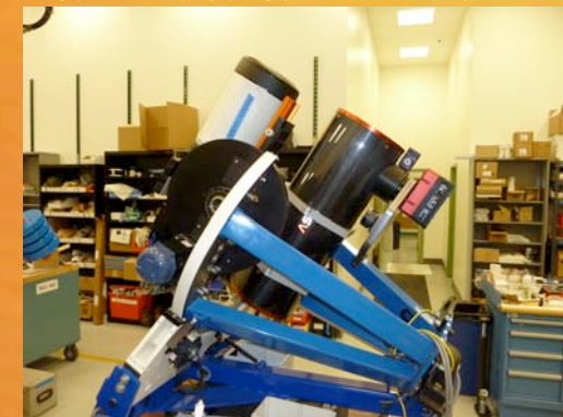
Production 1m assembly & testing for McDonald's (then CTIO) deployment. Note Baffles Astrograph Context & Deep Sky Spectrograph on 40cm mount. At least 1 per site.
