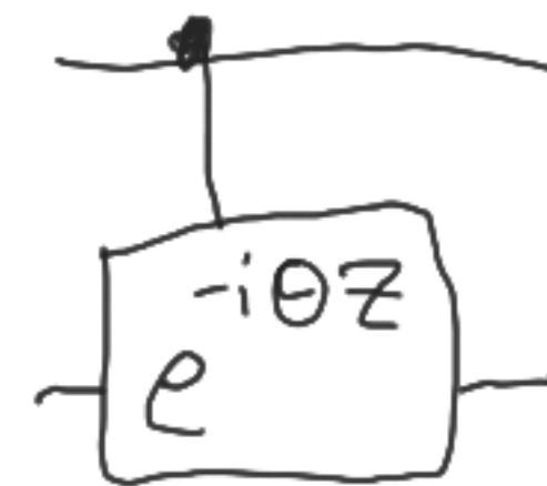
$$R_z(\phi) = e^{\frac{-i\phi}{2}Z} \quad \checkmark$$
