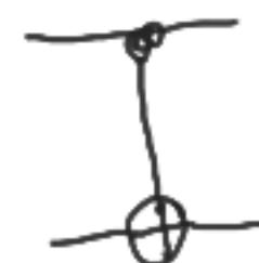
$$\begin{aligned}|00\rangle &\rightarrow |00\rangle \\|01\rangle &\rightarrow |01\rangle \\|10\rangle &\rightarrow |11\rangle \\|11\rangle &\rightarrow |10\rangle\end{aligned}$$
