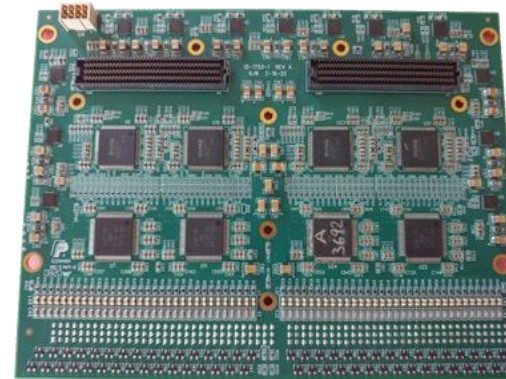
Analog Motherboard (P2 LArASIC + P1 ColdADC)
