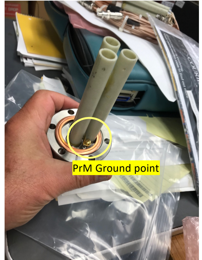
Underside of HV/Signal Feedthru
