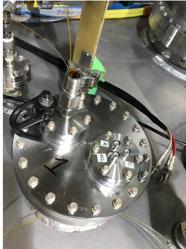
IB PrM Flange with HV/signal & Fiber Feedthrus
