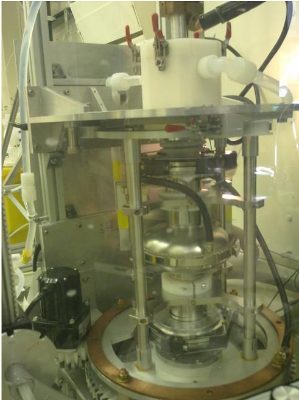
Draining of acid & rinsing after EP
