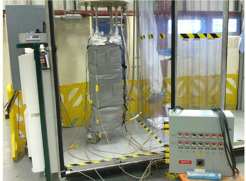
Heating Jackets around the cavity with temp monitor for 120 °C bake,
