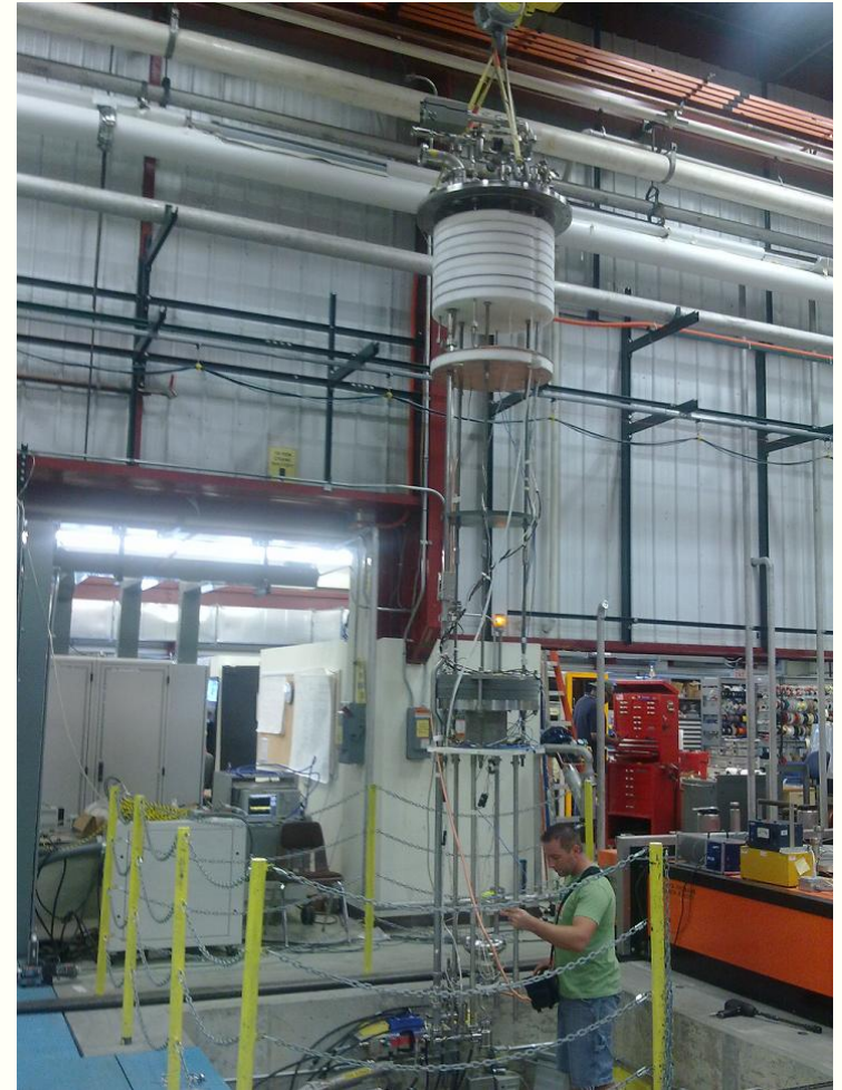
Cavity insert mounted inside the VTS cryostat
