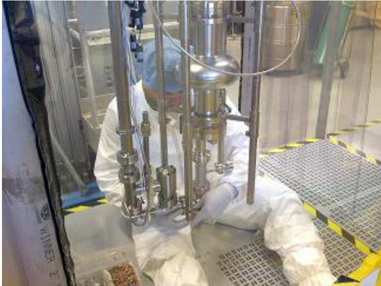
Assembly of cavity with VTS insert
