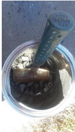
Sample #2 during crushing operation.
