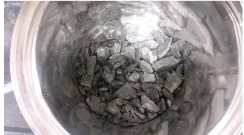
Sample #2 crushed to size for milling.
