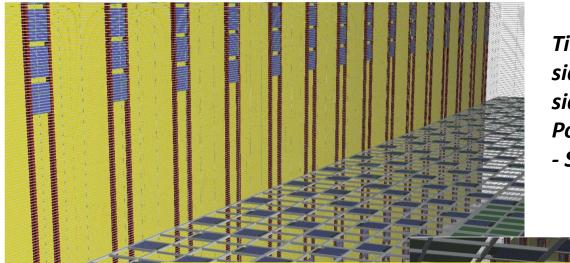
Tiles on the cathode are double sided -> have dichroic filters on both sides. Biased (Power over fiber - PoF) and read-out (Signal over fiber - SoF) through optical fibers.
