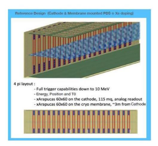
PD Active optical coverage on 3 sides: Cathode (sitting at high voltage) + long sides of the Cryostat walls (at ground)
