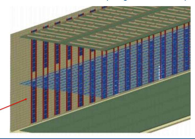
20 columns of 18 tiles (9 in top Drift region, 9 in bottom Drift region-- 720 total PD Modules)
