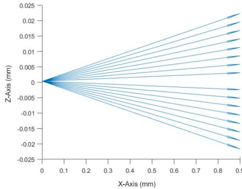
*Figure 9. SSR2 Cavity Beam Axis Vectors, Each Vector Representing the Position Of The Beam Axis After Set Screw B or C Have Been Given One Full Turn*
