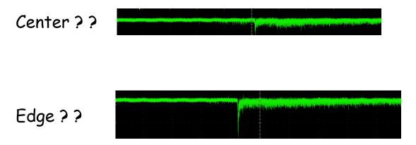
We can measure the discharge rate from the rf waveform - and infer a radius.
