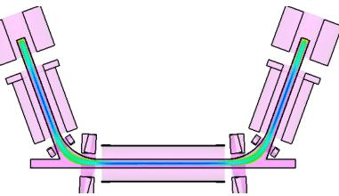
Conceptual design of the full magnetic system for the IOTA e-lens. Compared resistive and superconducting options.
