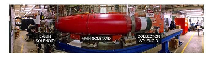
Started tests of existing 10-mm Gaussian electron gun (1.6 A at 10 kV), reused from the Tevatron, for the IOTA research program (Banerjee, Cathey, Stancari)
