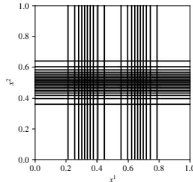
VEGAS grid for  $\int_0^1 d^4x \left( e^{-100(\vec{x}-\vec{r}_1)^2} + e^{-100(\vec{x}-\vec{r}_2)^2} \right)$
