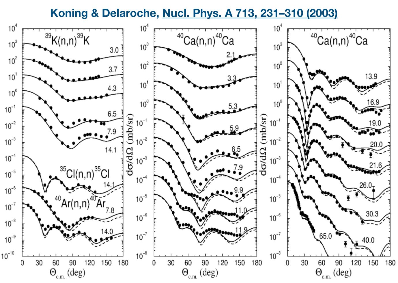
Dashed line is the global optical model fit that MARLEY currently uses. Solid lines are local fits to specific nuclei.
