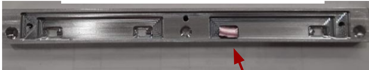
4-SiPM Fiber-Mating-Bar with 1 3D printed mockup of SiPM+carrier
