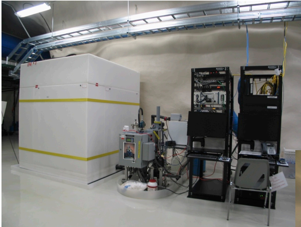
COUPP-4 bubble chamber, showing water tank shielding stack, pressure carts, DAQ racks
