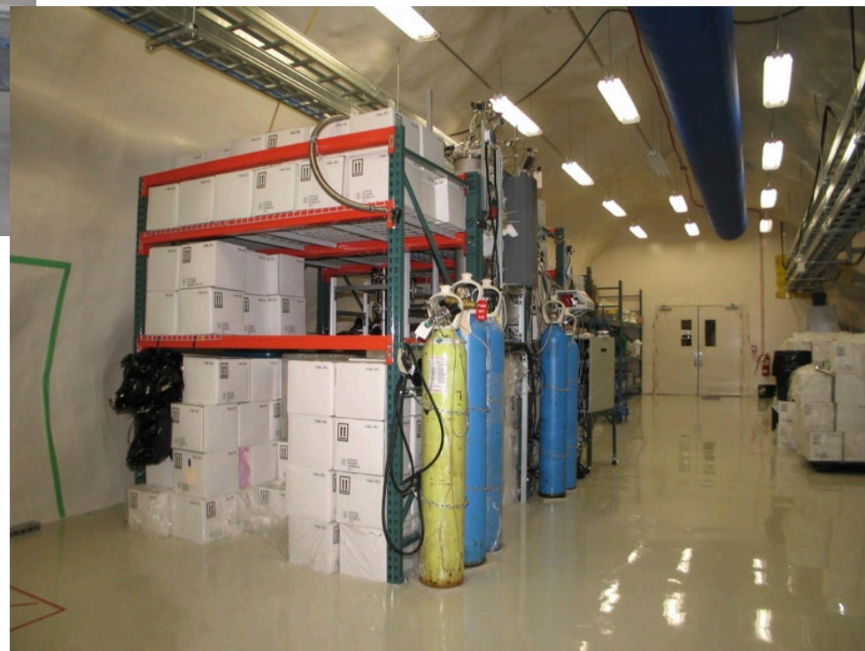
DEAP-I in the 'J'-Drift, showing water cube shielding and purifier stack
