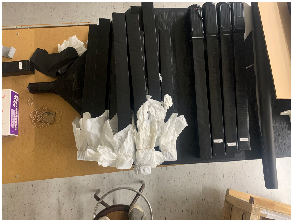
Scintillator bars and PMTs are wrapped together in Tyvek to maximise light collection efficiency.
