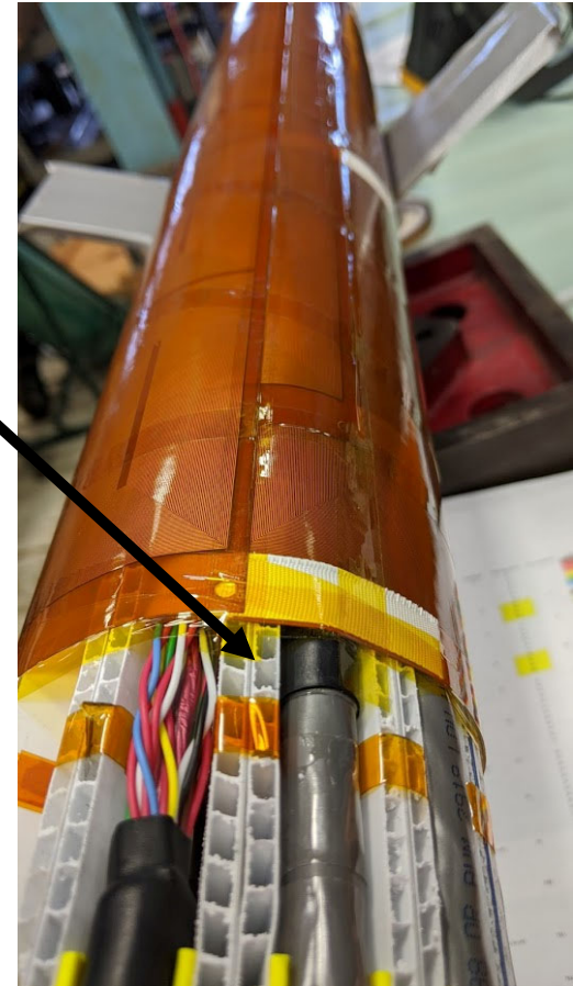
Theta detection with 12, full-length DQBuck radial circuits Positioned every 30 degrees.
