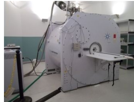
9.4 T human MRI @ UIC https://meml.lab.uic.edu 10.5 Tesla/88 cm bore Passively Shielded
