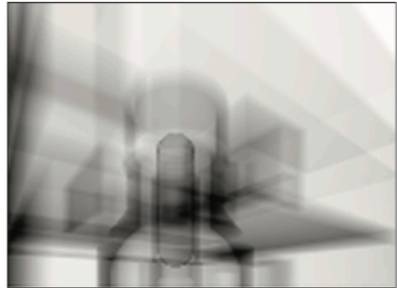
Muon scanning at Fukushima
