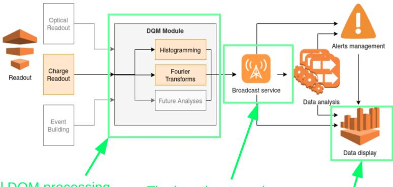
The local DQM processing module is designed to run an arbitrary number of algorithms in parallel over data from different sources.
