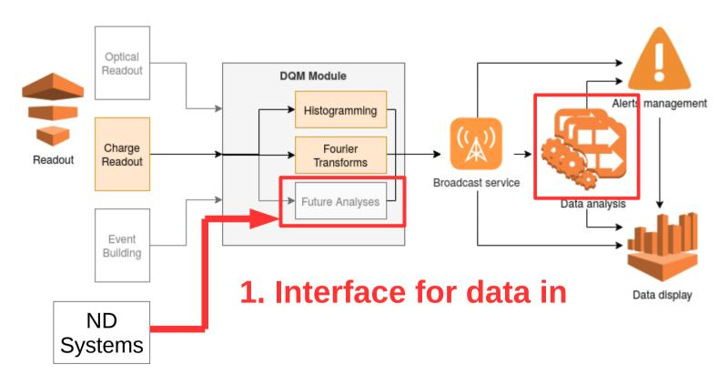
We are already set up to sample data from different sources at different, configurable rates – we just need a way for the systems to exchange requests and data packets. For the FD this is done with queues.
