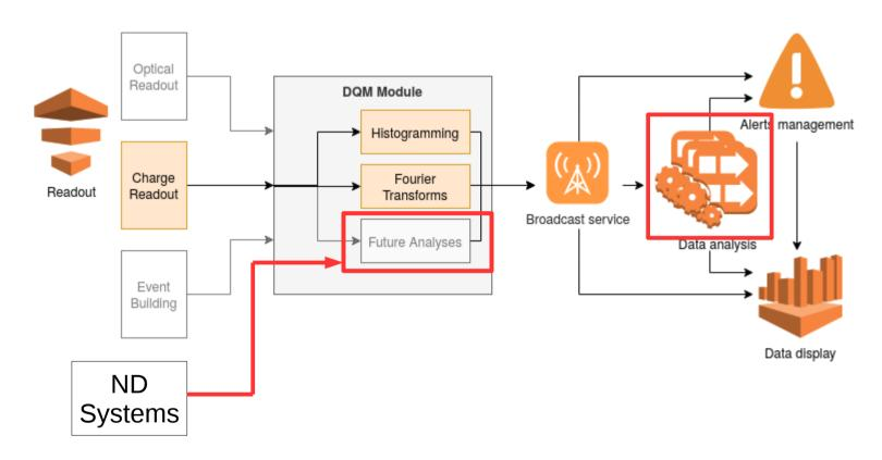
To use an instance of the DQM for the ND DAQ, these are the parts of the system that need extension/development.
