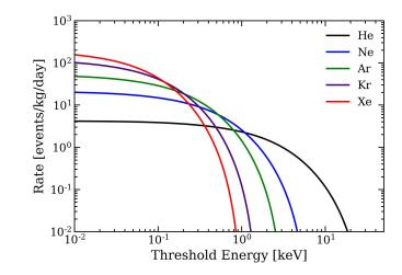
Integrated rate above threshold with  $6x10^{12}$  neutrino/cm<sup>2</sup>/s (25 m from 3 GWth reactor)
