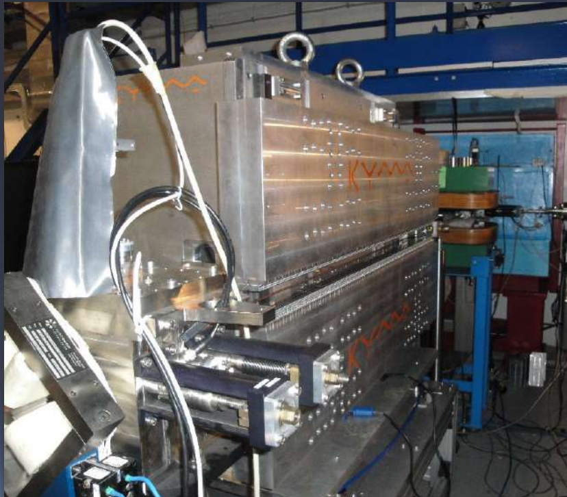
KYMA \Delta undulator at SPARC LAB: \lambda=1.4 cm, K1
