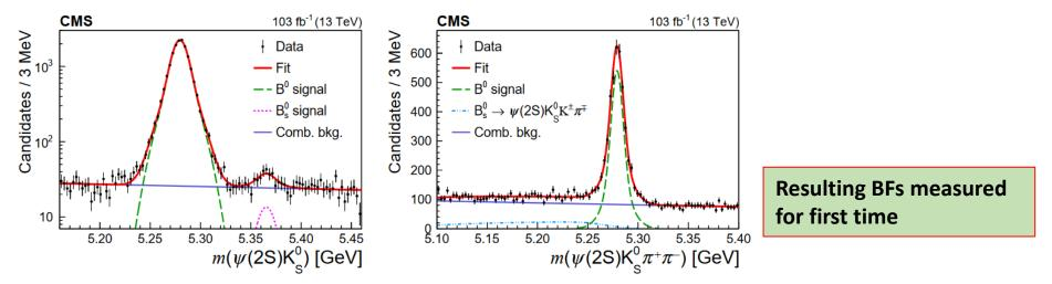
$\textit{B}(\text{Bs}^{0} \rightarrow \psi(2\text{S})\text{K}_{\text{S}}^{0}) / \textit{B}(\text{B0} \rightarrow \psi(2\text{S})\text{K}_{\text{S}}^{0}) = (3.33 \pm 0.69 \text{ (stat)} \pm 0.11 \text{ (syst)} \pm 0.34 \text{ (fs / fd ))} \times 10^{-2}$
