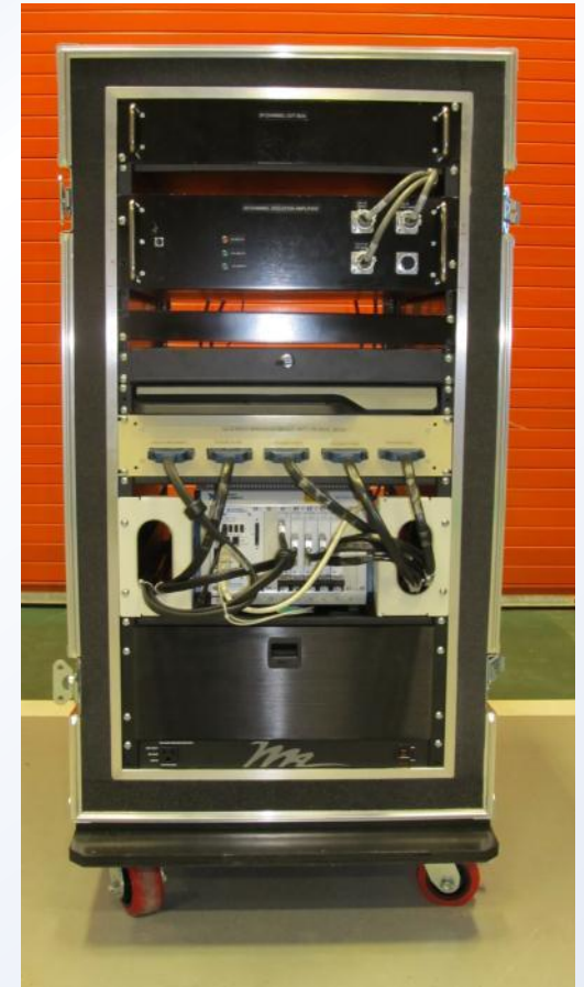
Quench Detection & Characterization DAQ Rack for the MICE Spectrometer Solenoid
