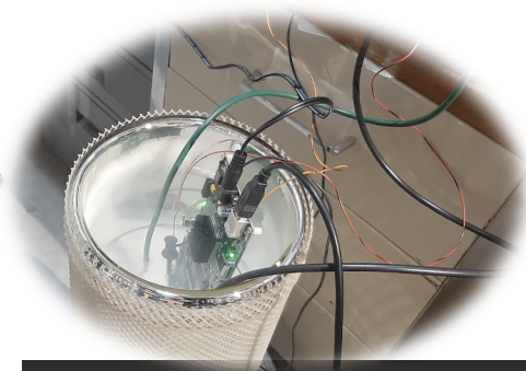
DUNE Cryogenic testing of digital and analog readout electronics at PAB
