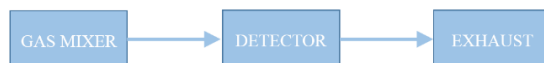
Figure 4.1: Schematic view of the simplest possible gas system: in open mode operation the gas mixture is vented after being used in the particle detector.
