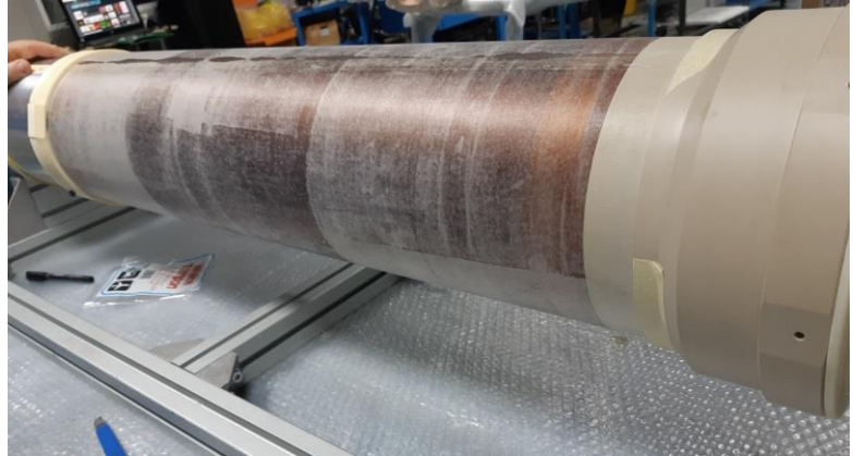
Figure 3.17: Fiberglass deposition on cathode.
