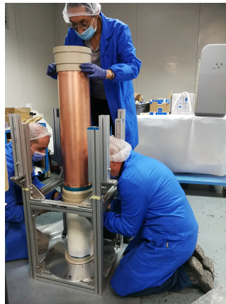
Figure 3.25: Assembly of the prototype. From top left: the cathode completed mounted on the assembly machine; the rectified millifoam support for the \mu -RWELL tiles; the manual insertion of the cathode on the cylindrical anode.
