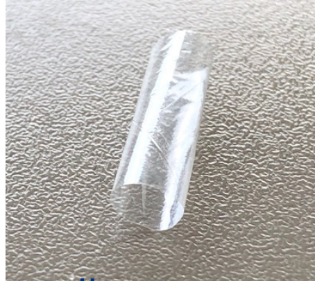
8 \mu m wall prototype straw
