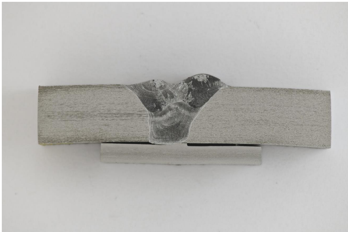
Figure 2, Macroscopic Appearance of Long MIG, 50% Hydrochloric Acid with Hydrogen Peroxide
