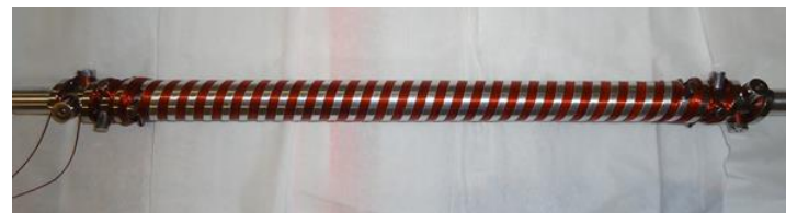
HSCU magnet core prototype.
