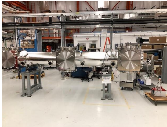
Cryostat vacuum vessel
