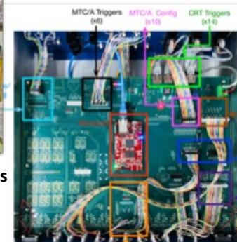
logic operations with the subsystem inputs send the information (timestamp + type of trigger + status) to the DAQ.
