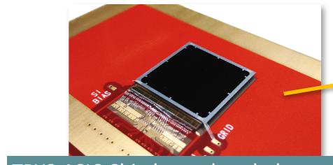
TPX3 ASIC Chip bump bonded to an optical sensor
