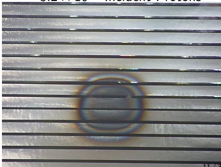
Upstream side after \sim 3.2 \times 10^{21} Incident Protons
