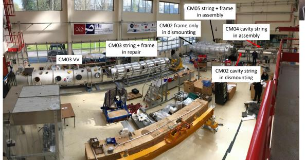
Spoke cryomodules at IJC-Lab
