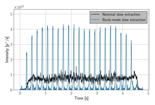
The spill profiles have been measured with a secondary emission monitor at the SPS.
