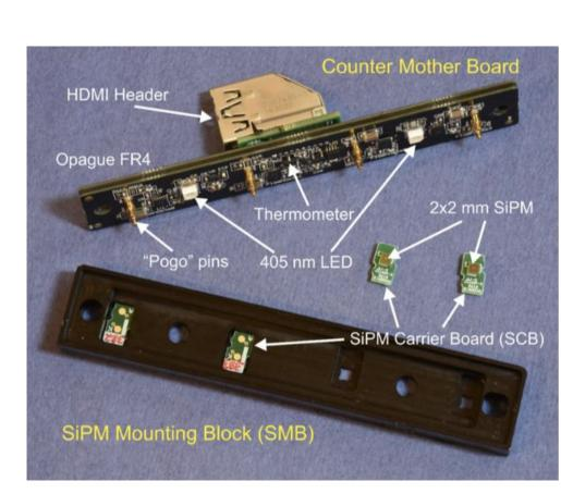
Components of the counter readout manifold.
