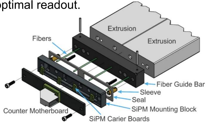
Blow-up of di-counter readout.
