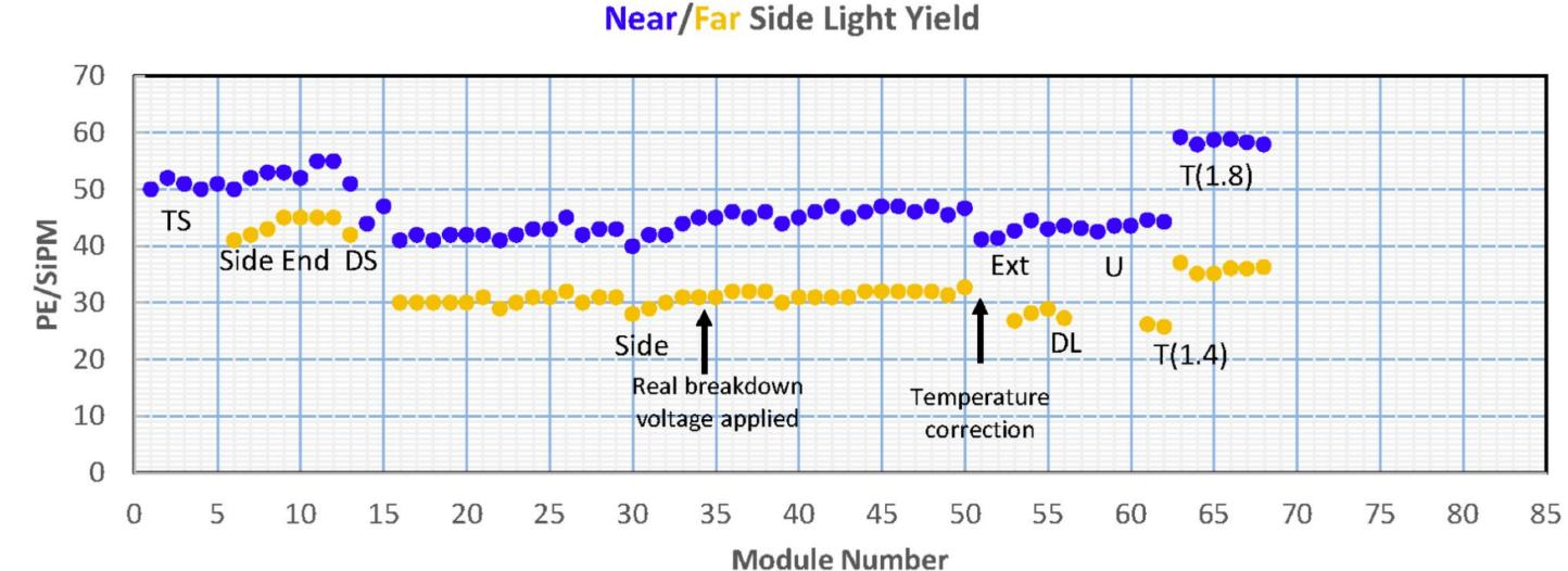
The average light yield (in units of photo-electrons) for all of the counters in each production module as measured using cosmic-ray muons.
