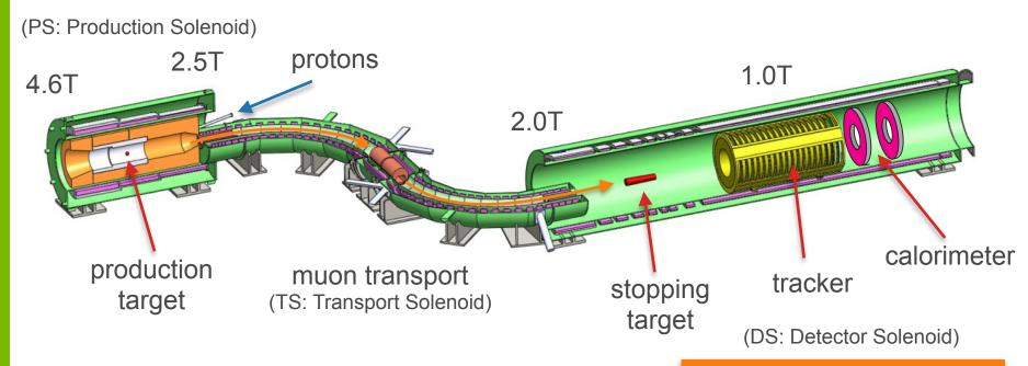
See talk 9: "Design, construction, and vertical slice performance tests of the Mu2e straw tracker", by Richard Bonventre
