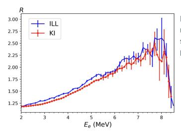
New <sup>235</sup>U/<sup>239</sup>Pu beta-decay spectral measurements at Kurchatov Institute suggest possible calibration issue with previous ILL measurements
