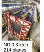
PVC extrusions filled with liquid scintillator(mineral oil + 5% pseudocumene)
