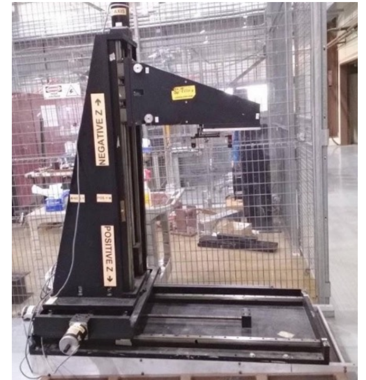
NuMI magnetic horn longitudinal field-mapping system
