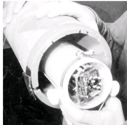
A robot camera developed by Todd Johnson and Duane Plant is inserted into the LCW system.
