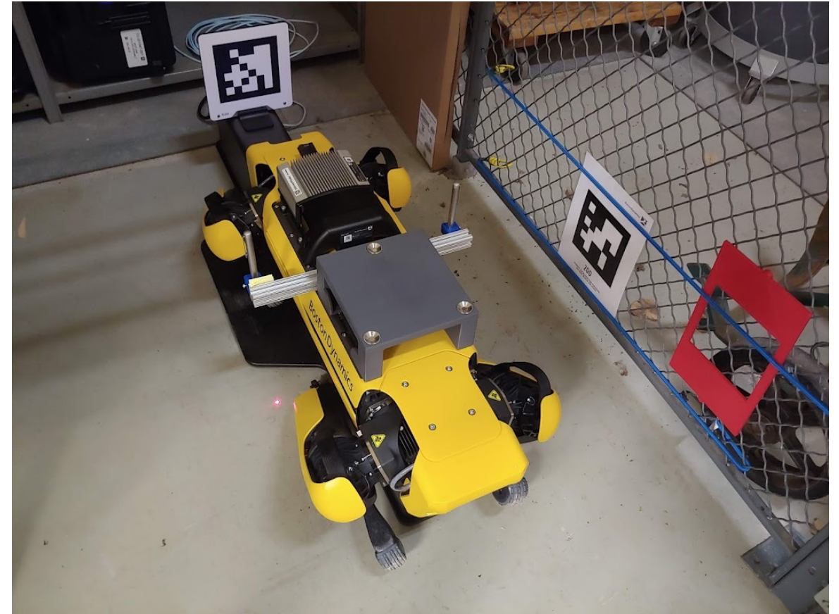
Spot on charging dock with localization test payload and nearby AprilTag fiducials
