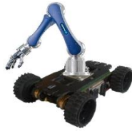
EXTRM robot with single arm (CERN made)
