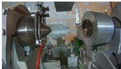
Temperature sensor installation on AD target
