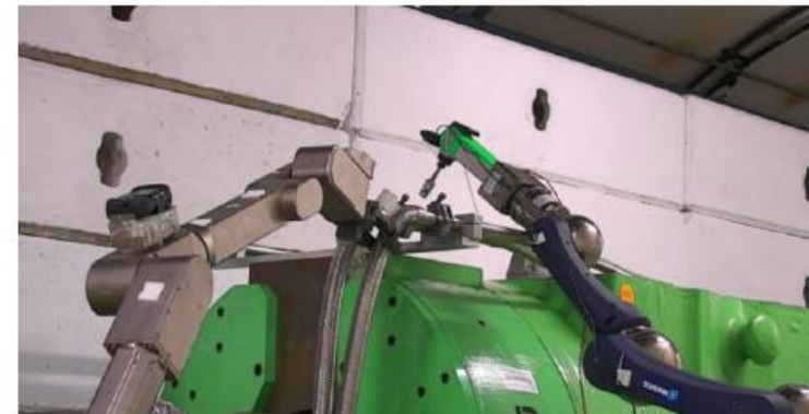
FIGURE 21. Robots in operation dismantling a beam dump water disconnection at CERN.
