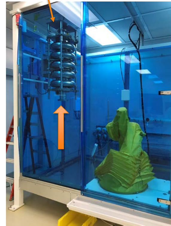
FRIB elliptical cleaning through one port
