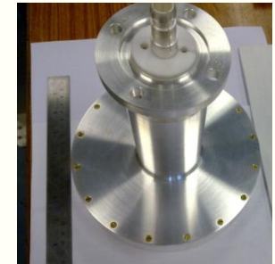
16-way 4kW Power combiner
