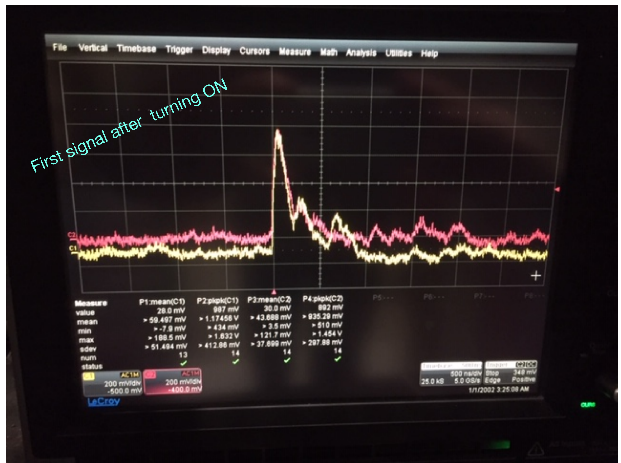
xARAPUCA Tile 2 channels - 80 SiPMs each (hybrid passive & active ganging)
