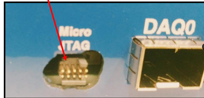
The JTAG Connector (Micro JTAG) is broken.
