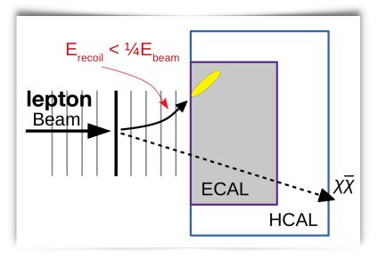
Dark matter events can be kinematically characterized by the calorimetric "disappearance" of a sizable fraction of the beam energy.
