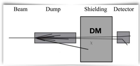
**Proton-beam** experiments are highly synergistic with the accelerator-based neutrino physics program. They use the same beamlines and detectors: LSND, MiniBooNE, COHERENT, CCM
