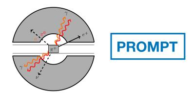
Production of an unstable dark sector particle from meson decay and detection of its SM decay products.
