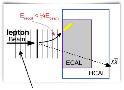
Dark matter events can be kinematically characterized by the calorimetric "disappearance" of a sizable fraction of the beam energy.
