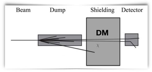
Production of dark matter in the dump and detection of its scattering in forward detectors.
