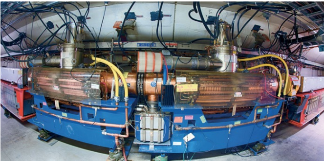
Booster 8 GeV Rapid-cycling synchrotron 0.5 km circumference
