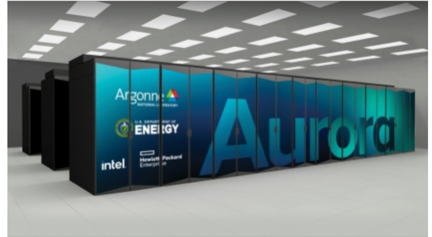
Aurora@Argonne: 20k CPUs 60k GPUs, 10PB memory, 2 DP exaflops
