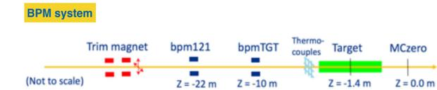
**BPM system,** displaying two of the bpm's monitoring the position of the proton beam before it collides with the target. **Left Middle:** The stripline bpm. The proton beam enters and passes through the stainless steel cylinder, causing electrons to congregate at the areas of highest positive charge density. The BPMs are fixed with ceramic supports, highlighted in green.
