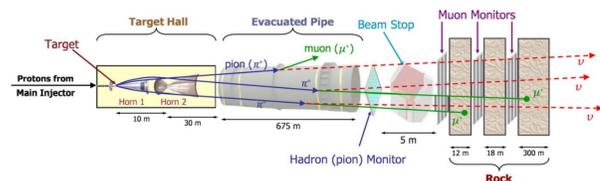
**NuMI Beamline System.** Protons exit the main injector and enter the target hall, where they collide with the target producing pions, which then decay into muons and muon neutrinos.
