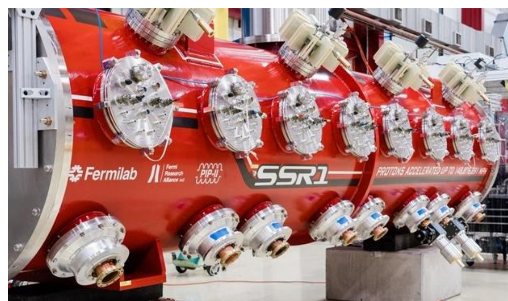
The first SSR1 cryomodule, which includes accelerator cavities and magnetic lenses, all cooled to 4K.
