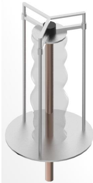
Figure 4: Bellows and legs concept, with motor (black) outside vacuum and flexible vacuum bellows shown as translucent.
