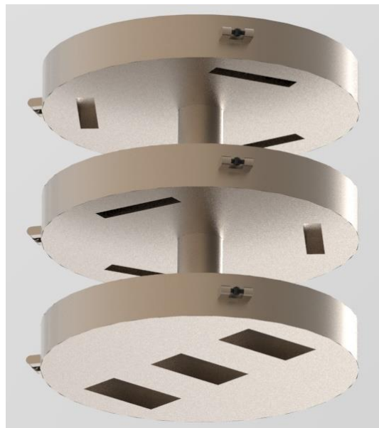
Figure 2: A rendering of the probe head concept. Slots represent Hall probes in different orientations.
