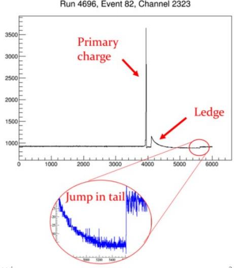
• The problem was reproduced in the laboratory both at LN2 temperature and at room temperature. It was traced to a network designed to improve the return-to-baseline performance of LArASIC relative to the version used for MicroBooNE. The parasitic gate capacitance of large transistors used in that "adaptive continuous reset" network reduced the loop stability of LArASIC and resulted in the ledge effect. This problem was eliminated for LArASIC\_P4.
